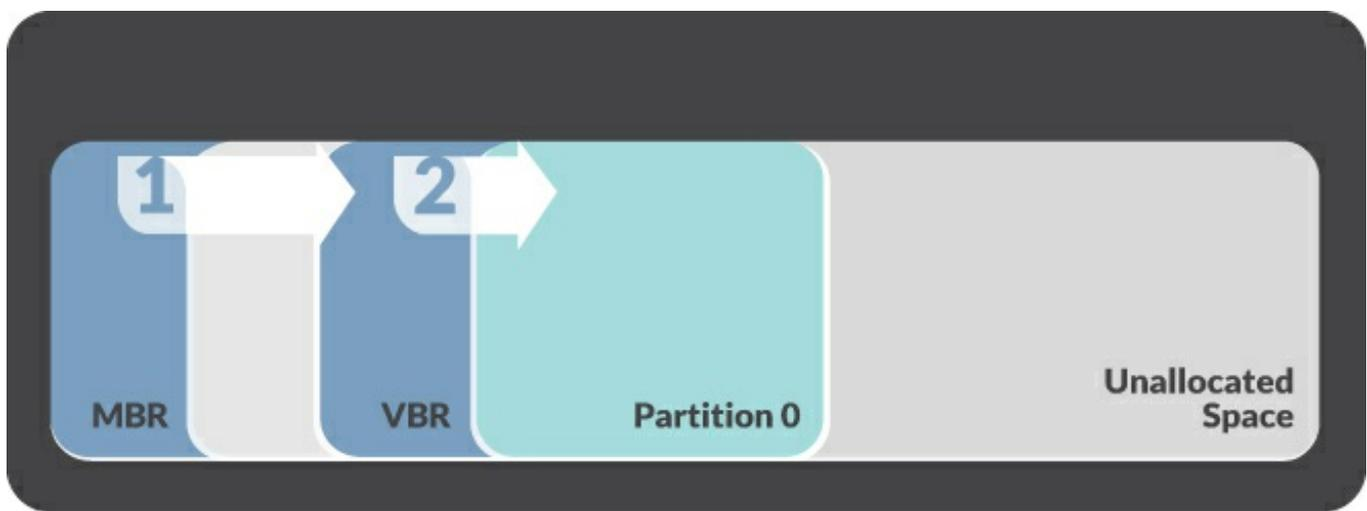
Figure 1. Simplified normal boot process
