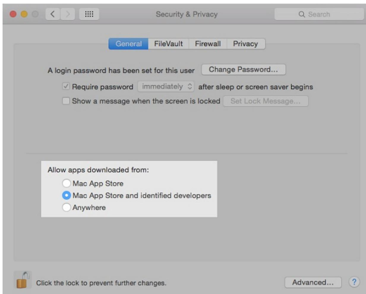
Figure 5. OS X can be configured to only permit trusted apps to execute
