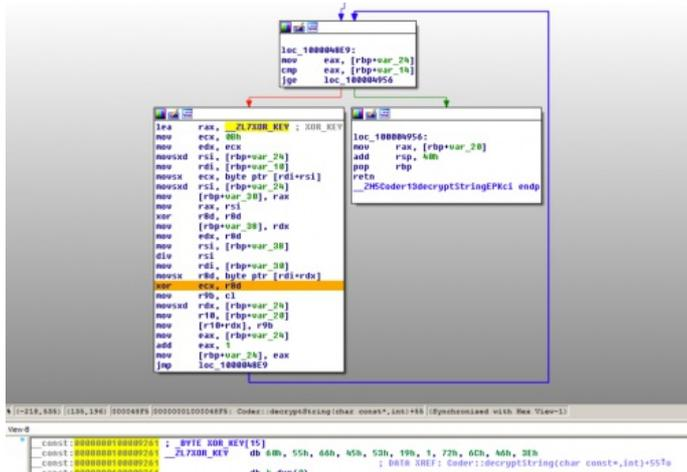
Figure 8 11-byte XOR algorithm used by Komplex to decrypt configuration strings
