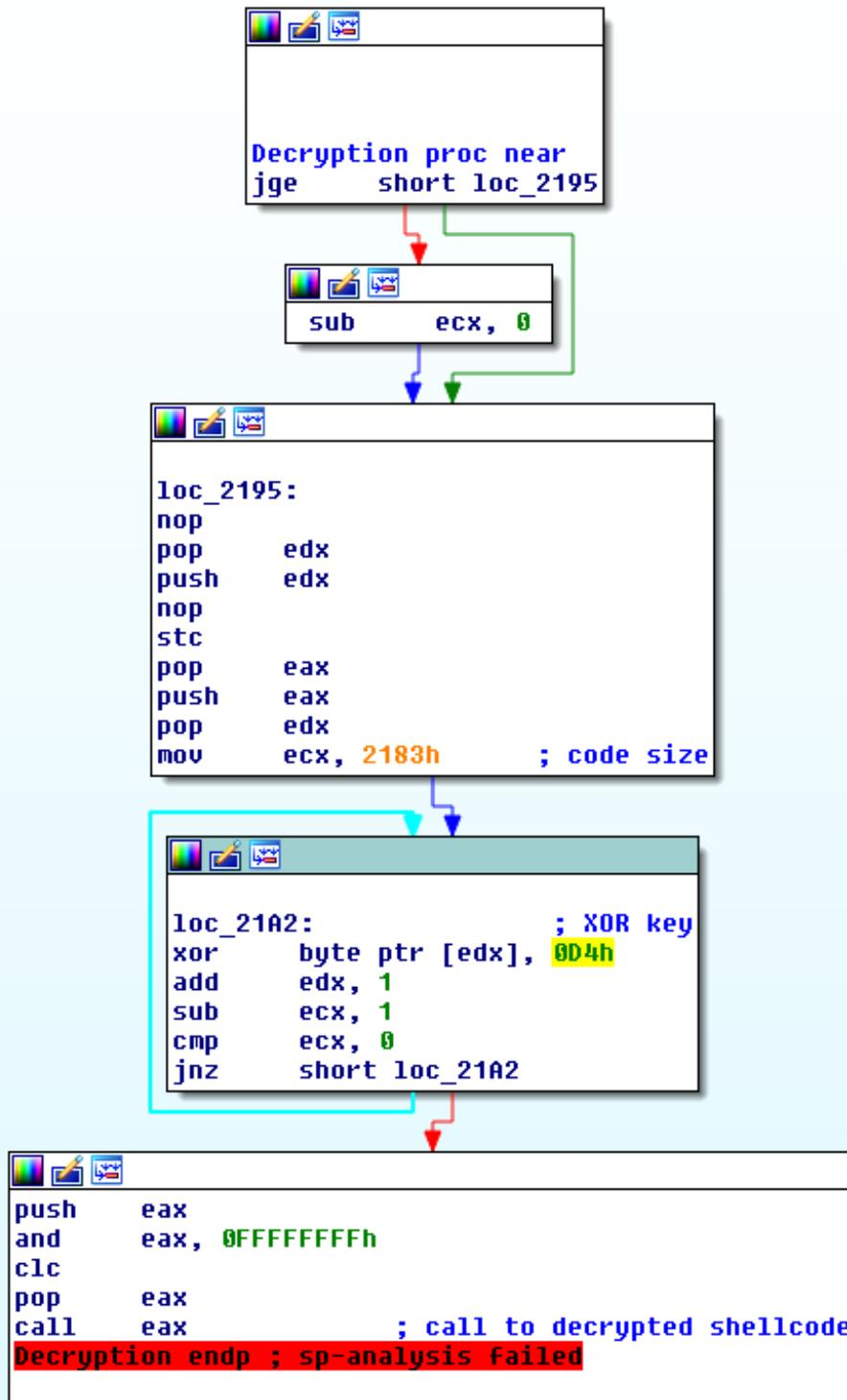
Figure 13: Decryption loop and call to decrypted shellcode
