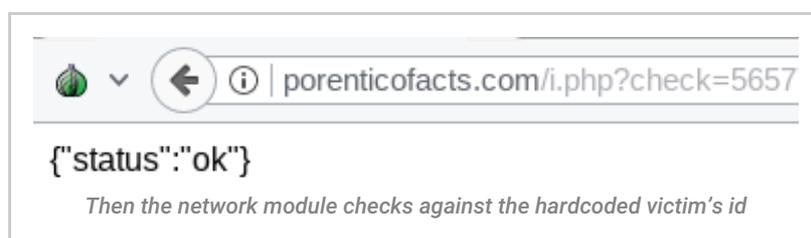
The network module checks against a 32-digit hardcoded victim id and sends the gathered data to the C2 using a HTTP POST request. In terms of programming, this id is strange, because the malware simultaneously 'fingerprints' its victim with an MD5 hash of its system data.
