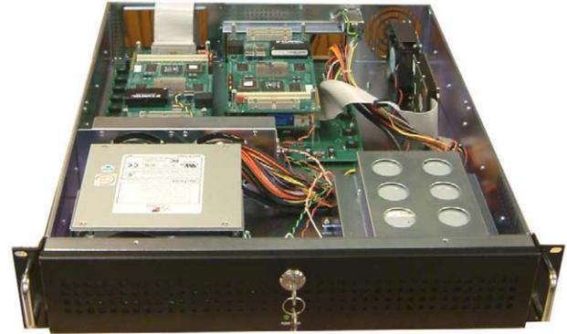
**Figure 4: Rackmount case holds DED with FPX cards**
